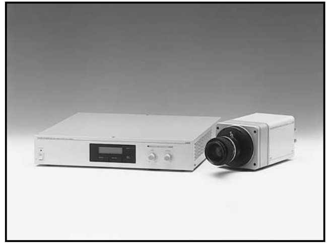
▲ Hermetic vacuum sealed water-cooled head type
