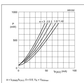
Fig.3 Maximum steady state power dissipation (forward plus leakage losses) as a function of average forward current.
