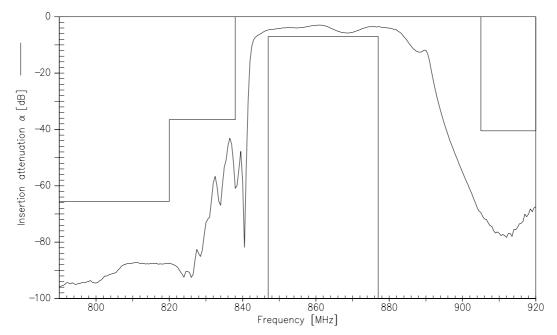
Measured transfer function(wideband, 2 filters B4114 in cascade without parallel coupling coil):
