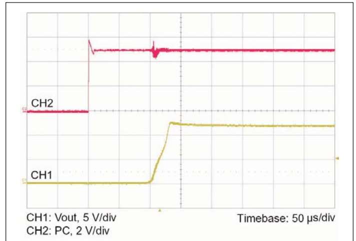
Figure 2 — Output voltage turn-on waveform with PC enabled at full load and 48 Vin
