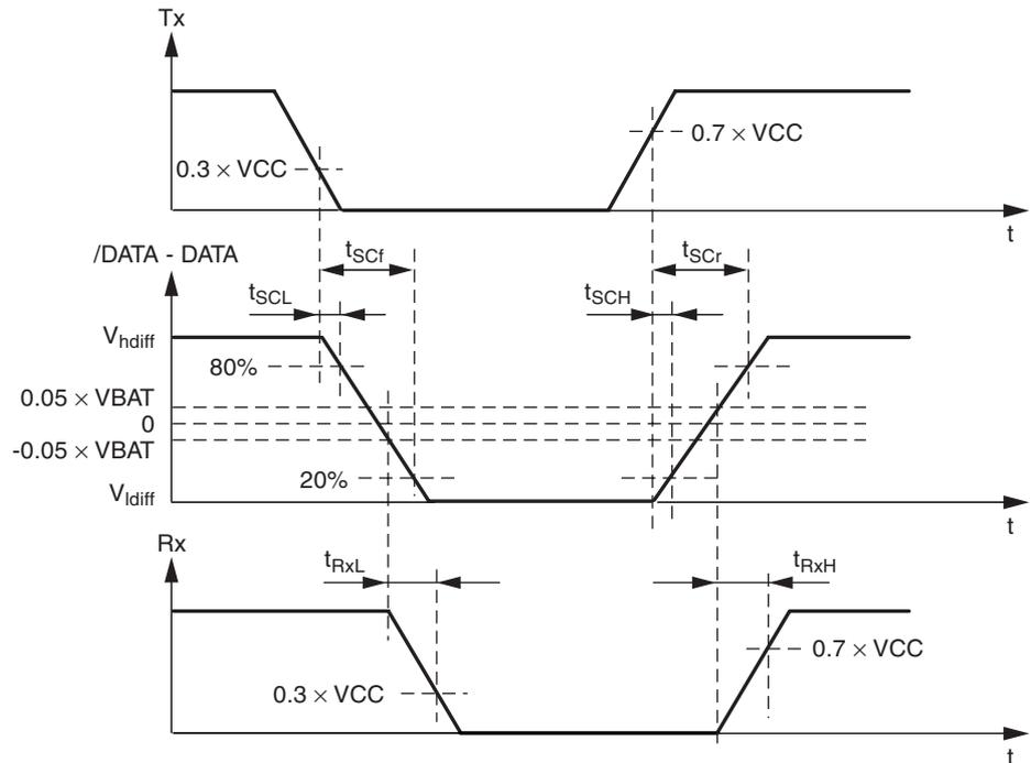
$$V_{\text{hdiff}} = V_{\text{VBAT}} \text{ (SCI driver is passive, recessive mode)}$$
