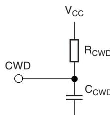
**Table 3-1.** Examples of Watchdog Oscillator Period  $t$  ( $\mu\text{s}$ ) as a Function of  $C_{\text{CWD}}$  and  $R_{\text{CWD}}$
