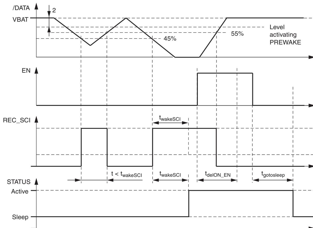
The status PREWAKE is characterized by the activated receive block of SCI and activated comparator of EN input. After going to Active, the  $V_{CC}$  regulator starts working. “Go to Sleep” is possible via a valid HIGH to LOW transition at pin EN (remaining LOW for longer than  $t_{gotosleep}$ ), if EN was previously in a valid HIGH state (HIGH for longer than  $t_{delON\_EN}$ ).
