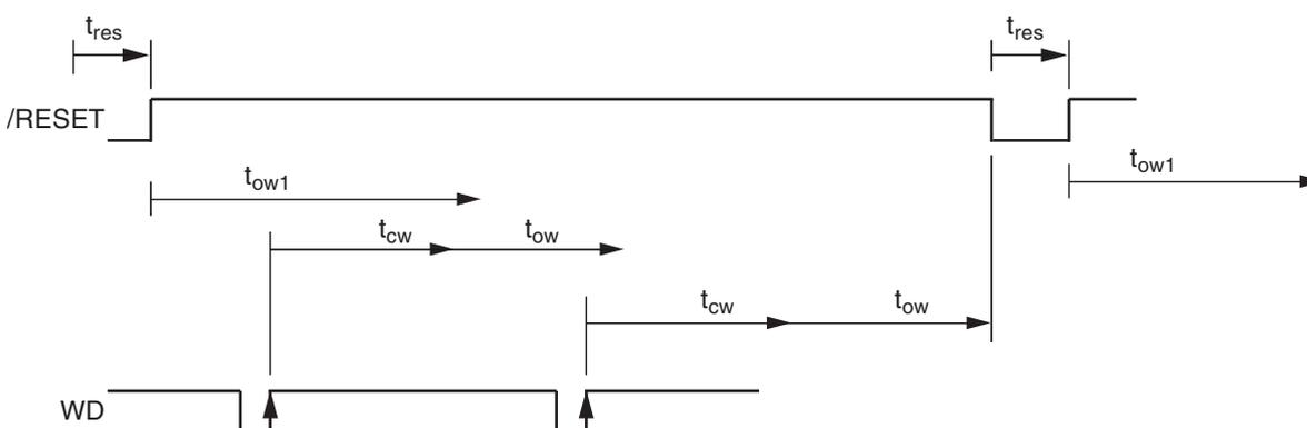
Figure 3-5. External Elements of the Watchdog
