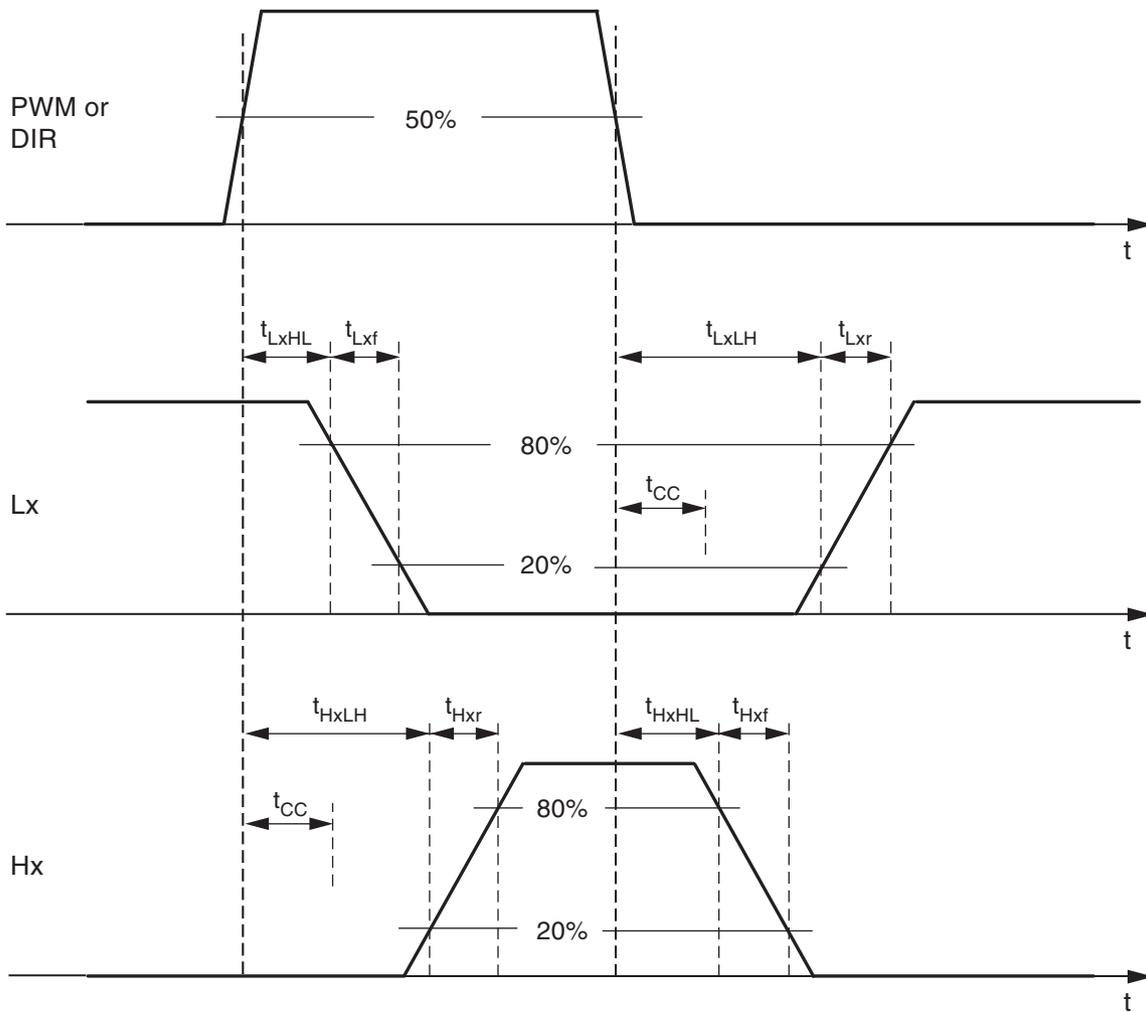
The delays  $t_{HxLH}$  and  $t_{LxLH}$  include the cross conduction time  $t_{cc}$ .
