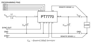
$\begin{array}{ll} C_{in} &= Required\ 2400\mu F\ electrolytic \\ C_{out} &= Required\ 2400\mu F\ electrolytic \\ L1 &= Optional\ 1\mu H\ input\ choke \end{array}$
