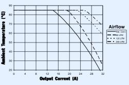
**Note A:** All characteristic data in the above graphs has been developed from actual procducts tested at 25°C. This data is considered typical for the ISR. **Note B:** OA curves represent operating conditions at which internal components are at or below manufacturer's maximum rated operating temperatures.
