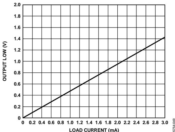
Figure 15. ALERT Output Low Voltage vs. Load Current
