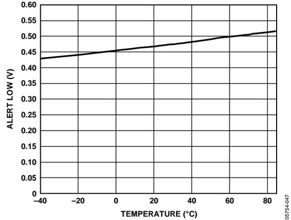
Figure 13. ALERT Output Low Voltage vs. Temperature @ 1 mA
