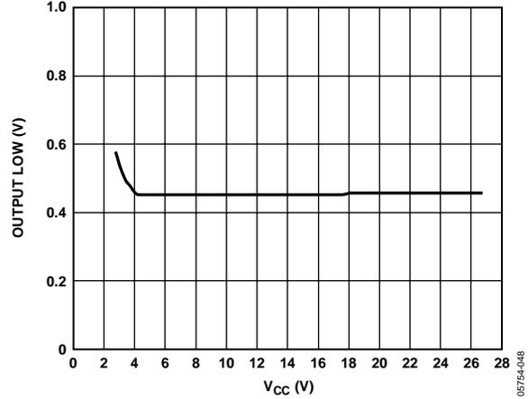
Figure 14. ALERT Output Low Voltage vs. Supply @ 1 mA
