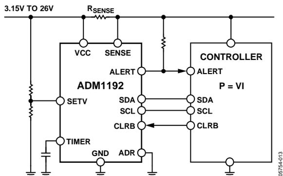
Figure 27. Using the ALERT Output as an Interrupt
