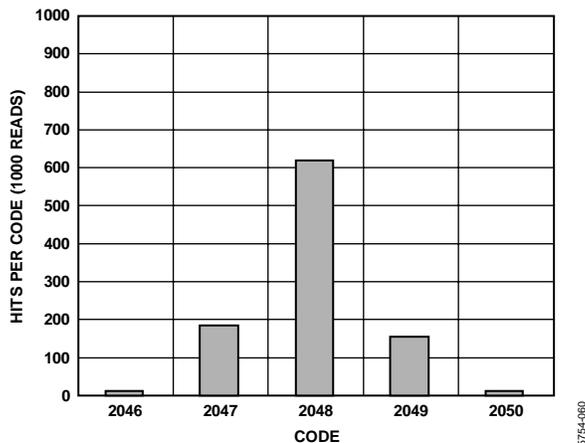
Figure 7. ADC Noise, Current Channel, Midcode Input, 1000 Reads
