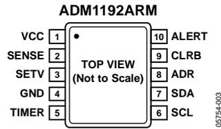
Figure 3. Pin Configuration
