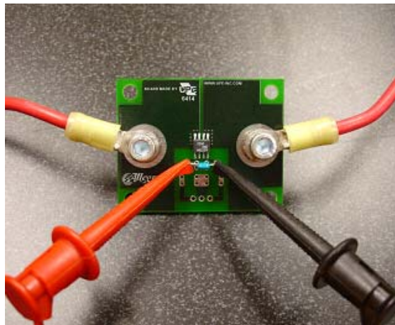
Allegro Current sensor evaluation board with ACS706 and external connections.
