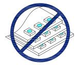
4. During surface-mounting, the pickup capillary diameter should be larger than the silicone lens to insure the capillary does not scratch or damage the lens.
