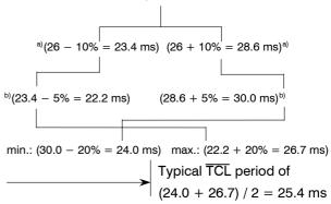
The ratio between  $T_{WD} = 26$  ms and the ( $\overline{TCL}$  period) = 25.4 ms is 0.975.
