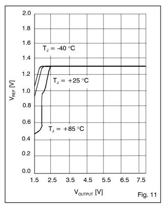
$V_{REF}$  versus  $V_{OUTPUT}$  at  $T_J$  = -40 °C, +25 °C, +85 °C
