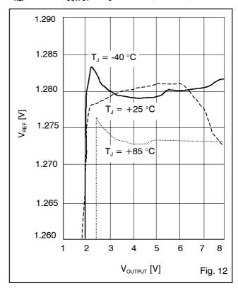
$V_{REF}$  versus Temperature at  $V_{OUTPUT}$  =3 V,5 V and 8 V  $V_{REF}$  versus Temperature at  $V_{OUTPUT}$  =3 V,5 V and 8 V
