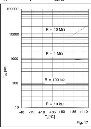
$T_{WD}$  versus R at  $V_{OUTPUT} = 5 V$
