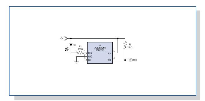
Figure 1. The MAX6316 μP supervisor monitors a fan's tachometer output.
