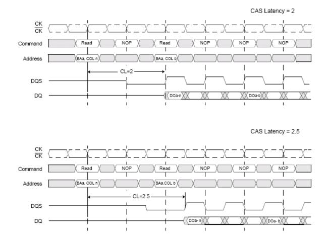
DO a-n (or a-b) = data out from bank a, column n (or bank a, column b).
