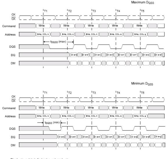
DI a-b, etc. = data in for bank a, column b, etc.
