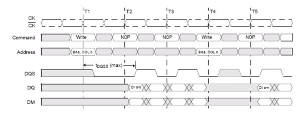
DI a-b, etc. = data in for bank a, column b, etc.
