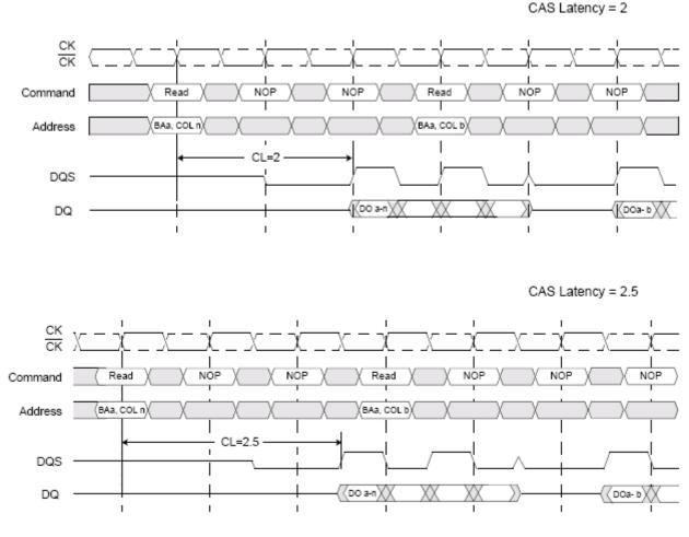
DO a-n (or a-b) = data out from bank a, column n (or bank a, column b). 3 subsequent elements of data out appear in the programmed order following DO a-n (and following DO a-b). Shown with nominal t<sub>AC</sub>, t<sub>DQSCK</sub>, and t<sub>DQSQ</sub>.
