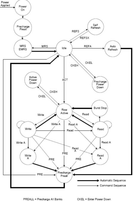
PREALL = Precharge All Banks MRS = Mode Register Set EMRS = Extended Mode Register Set REFS = Enter Self Refresh REFSX = Exit Self Refresh REFA = Auto Refresh CKEL = Enter Power Down CKEH = Exit Power Down ACT = Active Write A = Write with Autoprecharge Read A = Read with Autoprecharge PRE = Precharge
