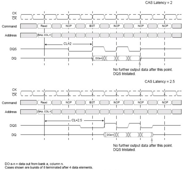
3 subsequent elements of data out appear in the programmed order following DO a-n. Shown with nominal  $t_{AC}, t_{\text{DQSCK}},$  and  $t_{\text{DQSQ}}.$
