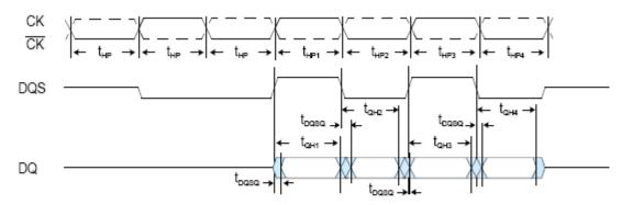
$t_{\rm HP}$  is the half cycle pulse width for each half cycle clock.  $t_{\rm HP}$  is referenced to the clock duty cycle only and not to the data strobe (DQS) duty cycle.
