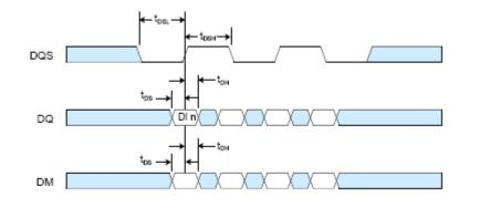
DI n = Data In for column n. 3 subsequent elements of data in are ar
