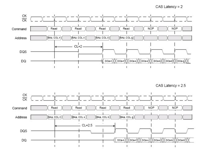
DO a-n, etc. = data out from bank a, column n etc. n' etc. = odd or even complement of n, etc. (i.e., column address LSB inverted). Reads are to active rows in any banks.
