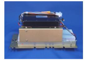
Mimix Broadband's SMaRTPAK (Standard Microwave Radio TWT replacement Power Amplifier Kit) amplifiers are uniquely designed to combine the DC/DC Converter, microwave amplifier and cooling devices into one single integrated unit. Each unit has been designed using modern device technology and includes reverse polarity, overvoltage and excess thermal protection. Unlike TWT's and other TWT replacement options, SMaRTPAKs do not require a separate, bulky and often unreliable power supply.
