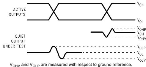
Input pulses have the following characteristics:  $f = 1 \text{ MHz}$ ,  $t_r = 3 \text{ ns}$ ,  $t_f = 3 \text{ ns}$ , skew  $< 150 \text{ ps}$ .
