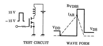
$$\begin{aligned} &RG = 25~\Omega \\ &V_{DD} = 25~V,~L = 371~\mu H \end{aligned} \qquad E_{AS} = \frac{1}{2} \cdot L \cdot I^2 \cdot \left( \frac{BV_{DSS}}{BV_{DSS} - V_{DD}} \right) \end{aligned}$$
