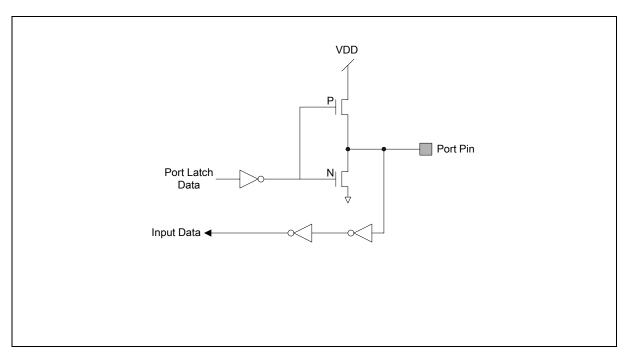
Figure 20-4: Push-Pull Output
