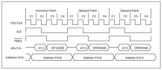
Figure 9-3: Three Cycles Instruction Timing
