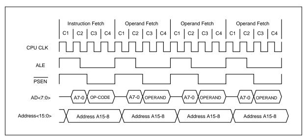
Figure 9-4: Four Cycles Instruction Timing
