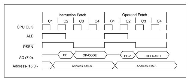
Figure 9-2: Two Cycles Instruction Timing
