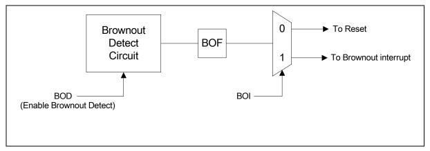
Figure 22-1: Brownout Detect Block
