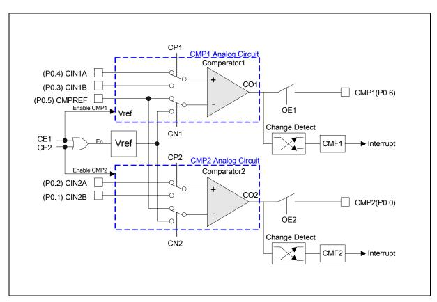
Figure 19-1: Analog Comparators
