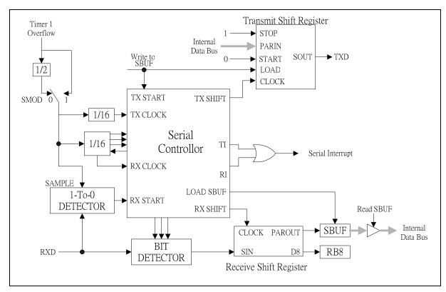
Figure 16-2: Serial Port Mode 1
