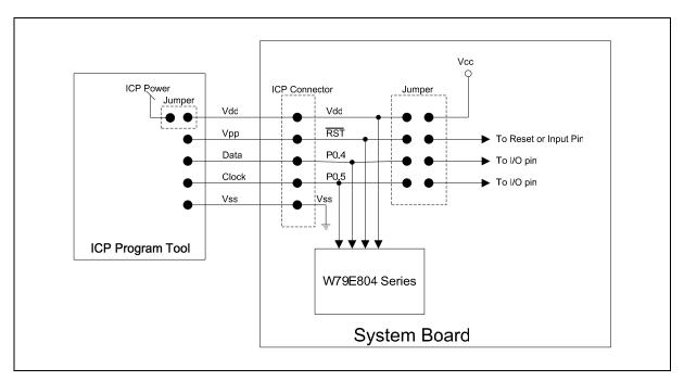
Figure 25-1: Application Circuit of ICP
