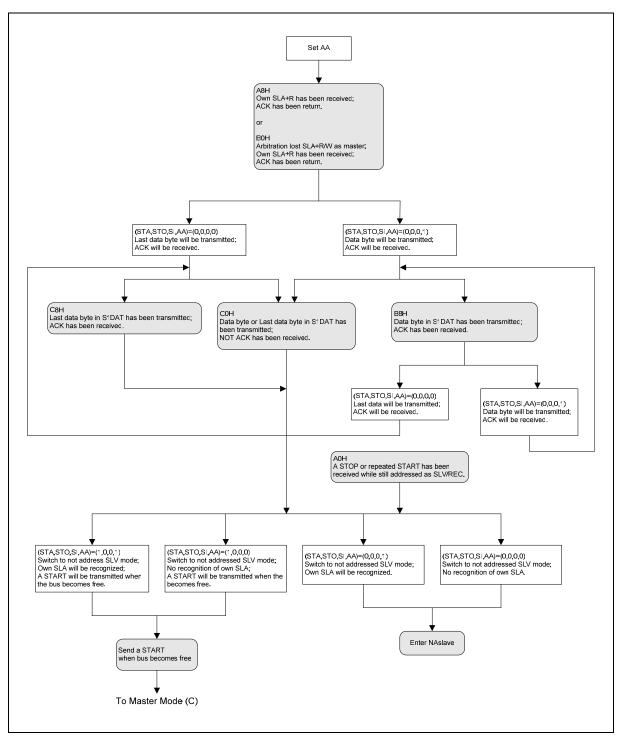
Figure 24-6: Slave Transmitter Mode
