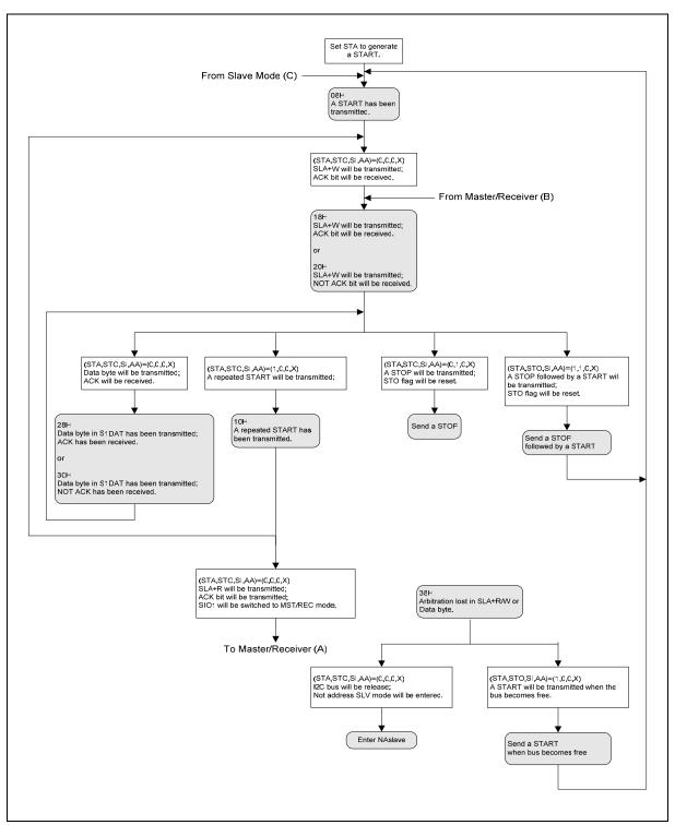
Figure 24-4: Master Transmitter Mode
