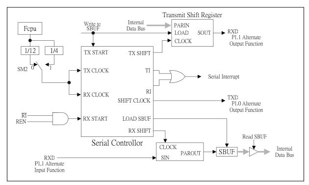
Figure 16-1: Serial Port Mode 0
