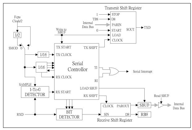
Figure 16-3: Serial Port Mode 2
