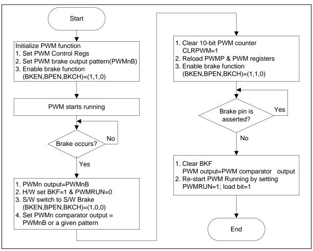
Figure 23-2: PWM Brake Function
