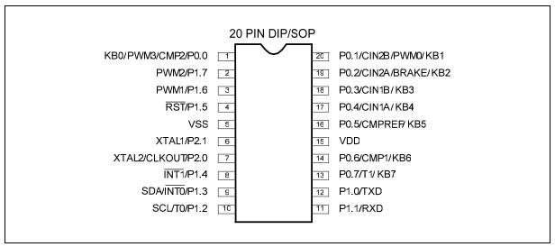
Figure 4-1: Pin Configuration
