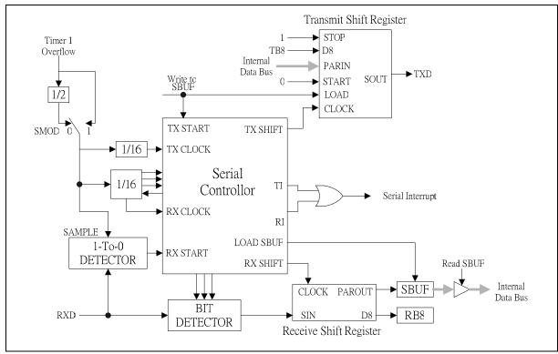
Figure 16-4: Serial Port Mode 3
