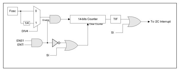
Figure 24-2: I2C Timer Count Block Diagram
