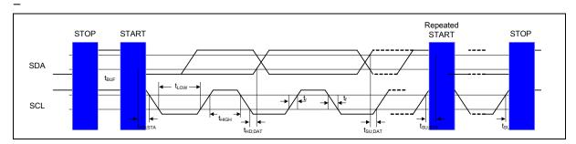
Figure 24-1: I2C Bus Timing
