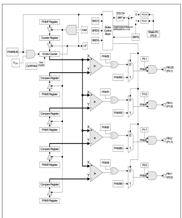
Figure 23-1: W79E804/803/802 PWM Block Diagram
