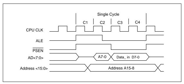
Figure 9-1: Single Cycle Instruction Timing
