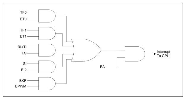
Figure 12-2: Interrupt Sources that cannot wake up from Power Down Mode
