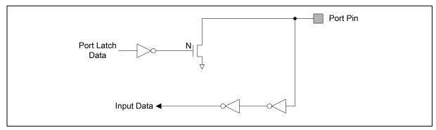
Figure 20-3: Open Drain Output
