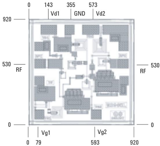
**Figure 20. AMMC - 5618 Bond pad locations**
