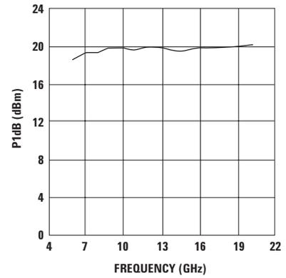
**Figure 6. output Power at 1 dB Gain Compression**
