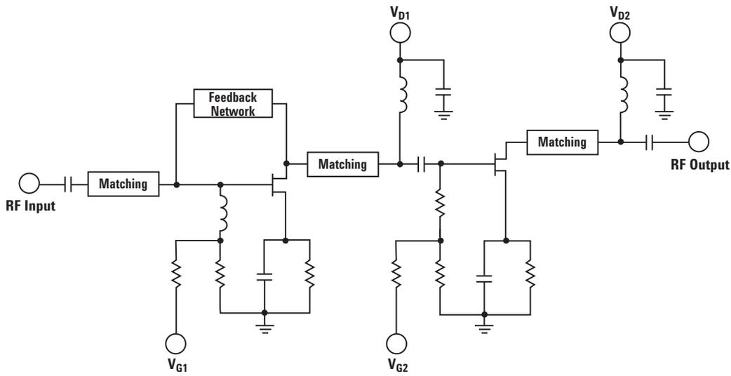
Figure 18. AMMC - 5618 Schematic
