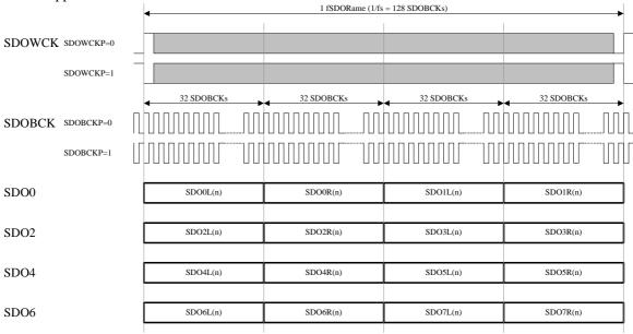
The TDM 8ch mode timing is illustrated below. 32-bit data can be output via the eight channels from SDO0 and SDO4.
