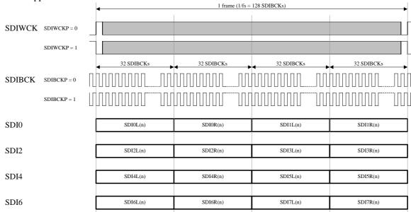
The TDM 8ch mode timing is illustrated below. 32-bit data can be input via the eight channels from SDI0 and SDI4. The supported data format is the same as for normal mode.
