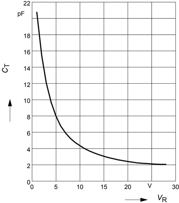
**Normalized diode capacitance**
