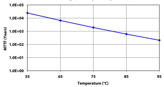
MTTF is calculated from accelerated life-time data of single devices and assumes isothermal back-plate.
