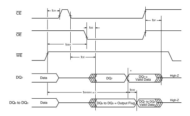
\*: DQ<sub>7</sub> = Valid Data (The device has completed the Embedded operation.)
