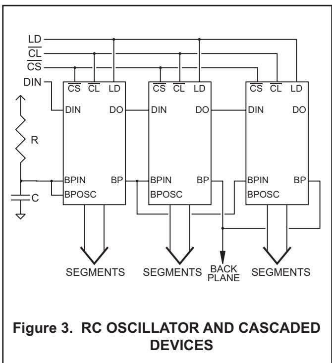
**Figure 3. RC OSCILLATOR AND CASCADED DEVICES**
