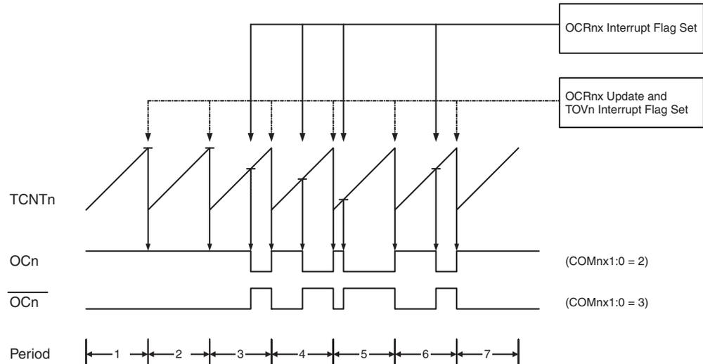
The Timer/Counter Overflow Flag (TOV0) is set each time the counter reaches MAX. If the interrupt is enabled, the interrupt handler routine can be used for updating the compare value.
