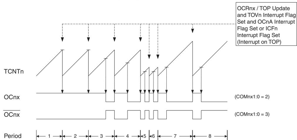
The Timer/Counter Overflow Flag (TOV1) is set each time the counter reaches TOP. In addition the OC1A or ICF1 Flag is set at the same timer clock cycle as TOV1 is set when either OCR1A
