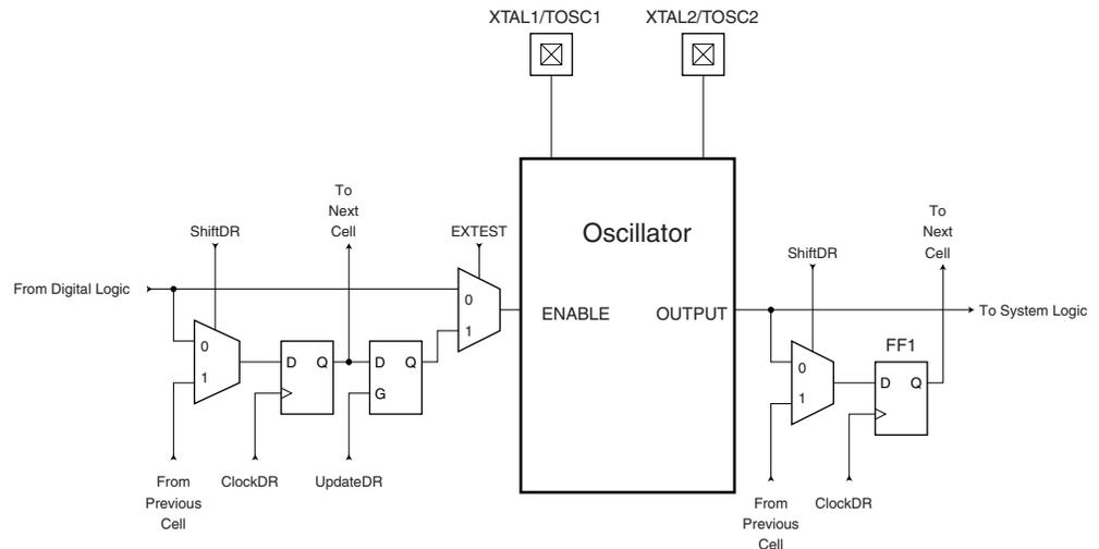
Table 24-1 summarizes the scan registers for the external clock pin XTAL1, oscillators with XTAL1/XTAL2 connections as well as 32kHz Timer Oscillator.
