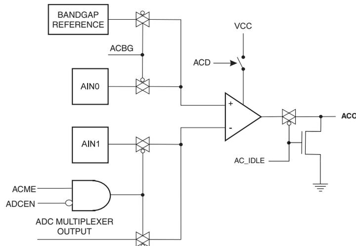
**Figure 24-8.** General Boundary-scan cell Used for Signals for Comparator and ADC
