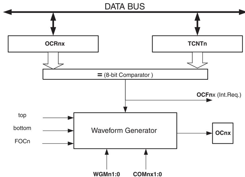
The OCR2A Register is double buffered when using any of the Pulse Width Modulation (PWM) modes. For the Normal and Clear Timer on Compare (CTC) modes of operation, the double buffering is disabled. The double buffering synchronizes the update of the OCR2A Compare Register to either top or bottom of the counting sequence. The synchronization prevents the occurrence of odd-length, non-symmetrical PWM pulses, thereby making the output glitch-free.
