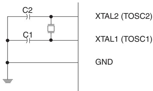
The Oscillator can operate in three different modes, each optimized for a specific frequency range. The operating mode is selected by the fuses CKSEL3:1 as shown in [Table 7-5](#).
