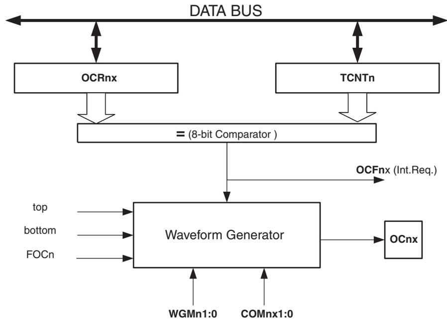
The OCR0A Register is double buffered when using any of the Pulse Width Modulation (PWM) modes. For the normal and Clear Timer on Compare (CTC) modes of operation, the double buffering is disabled. The double buffering synchronizes the update of the OCR0 Compare Register to either top or bottom of the counting sequence. The synchronization prevents the occurrence of odd-length, non-symmetrical PWM pulses, thereby making the output glitch-free.
