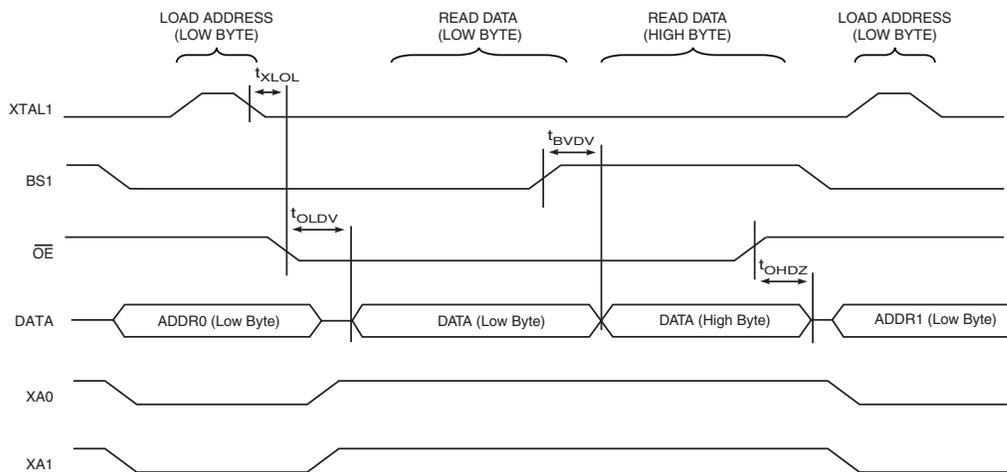
Note: 1. The timing requirements shown in Figure 26-7 (i.e.,  $t_{DVXH}$ ,  $t_{XHXL}$ , and  $t_{XLDX}$ ) also apply to reading operation.
