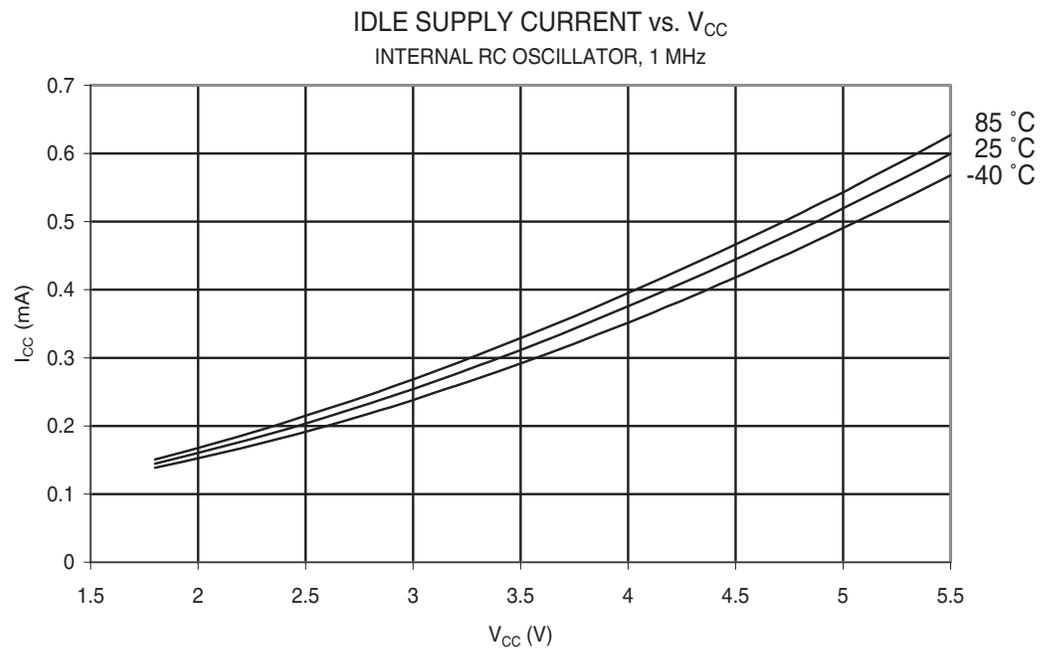
**Figure 28-10.** Idle Supply Current vs.  $V_{CC}$  (32 kHz Watch Crystal)
