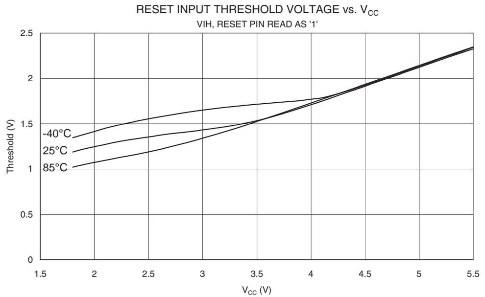
**Figure 28-46.** Reset Input Pin Hysteresis vs.  $V_{CC}$
