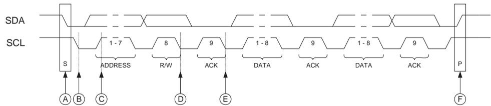
Referring to the timing diagram (Figure 19-5.), a bus transfer involves the following steps:
