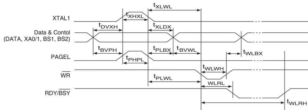
**Figure 26-8.** Parallel Programming Timing, Loading Sequence with Timing Requirements<sup>(1)</sup>
