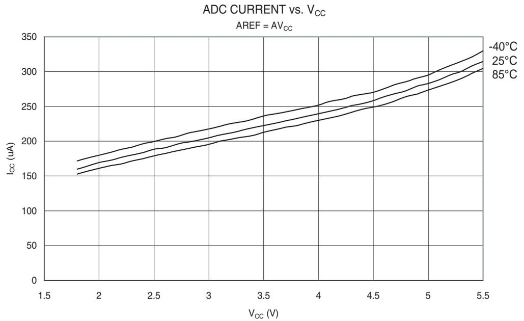
**Figure 28-60.** AREF External Reference Current vs.  $V_{CC}$
