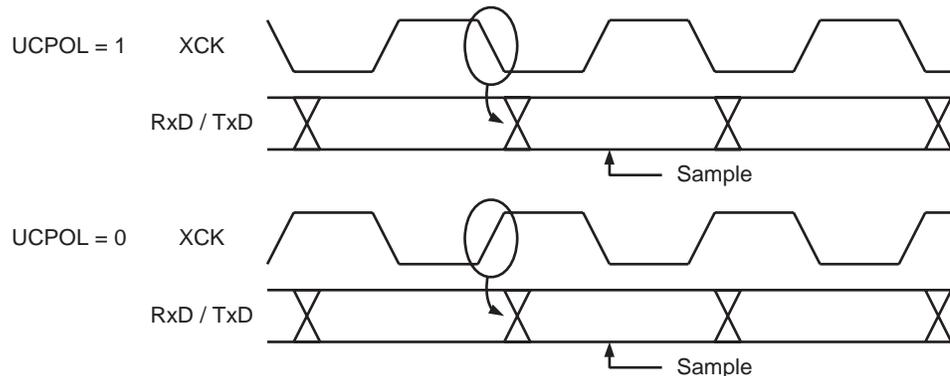
The UCPOLn bit UCRSC selects which XCK clock edge is used for data sampling and which is used for data change. As [Figure 18-3](#) shows, when UCPOLn is zero the data will be changed at rising XCK edge and sampled at falling XCK edge. If UCPOLn is set, the data will be changed at falling XCK edge and sampled at rising XCK edge.
