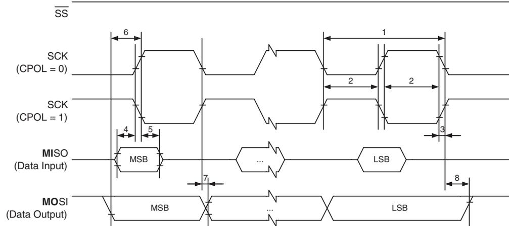
**Figure 27-5. SPI Interface Timing Requirements (Slave Mode)**
