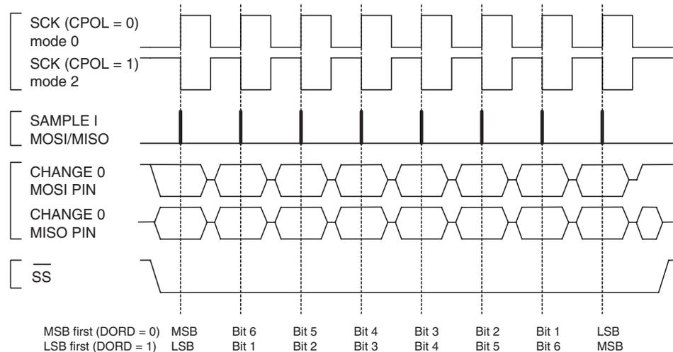
**Figure 17-4.** SPI Transfer Format with CPHA = 1
