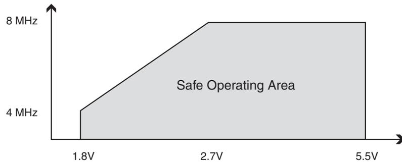
**Figure 27-2.** Maximum Frequency vs.  $V_{CC}$ , ATmega169P
