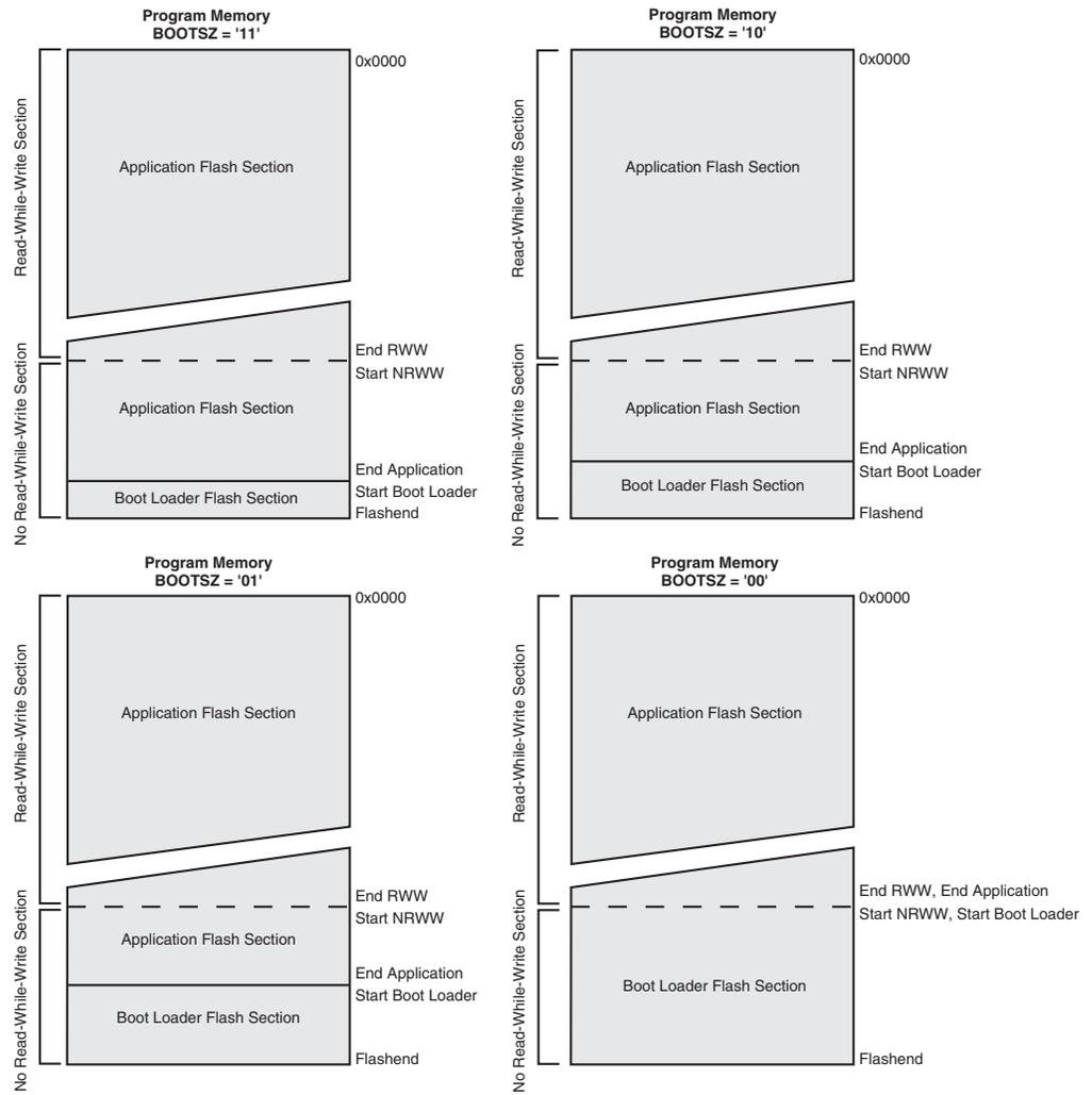
Note: 1. The parameters in the figure above are given in [Table 25-6 on page 289](#).
