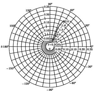
$\begin{array}{l} \text{S22e} \\ \text{VCE} = 5\text{V} \\ \text{IC} = 10\text{mA} \\ \text{Ta} = 25^{\circ}\text{C} \\ \text{(UNIT}: \Omega) \end{array}$
