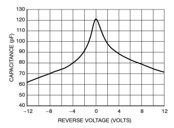
Figure 4. Typical Line Capacitance vs. Reverse Bias Voltage
