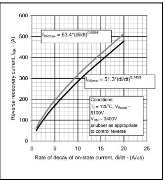
Fig.13 Reverse recovery current
