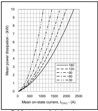
Fig.3 On-state power dissipation – sine wave
