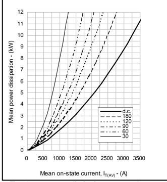
Fig.6 On-state power dissipation - rectangular wave
