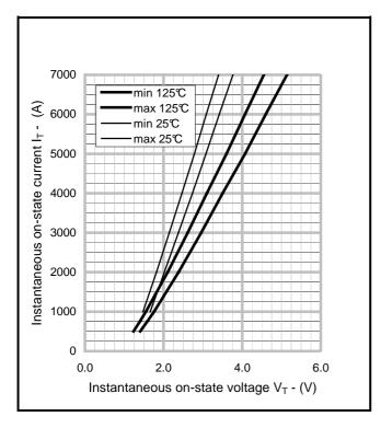
Fig.2 Maximum & minimum on-state characteristics
