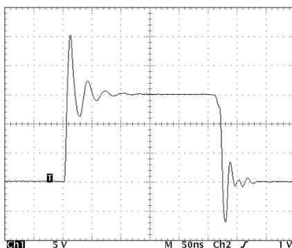
**Figure 6 - EVIC420 Typical Gate Waveform**
