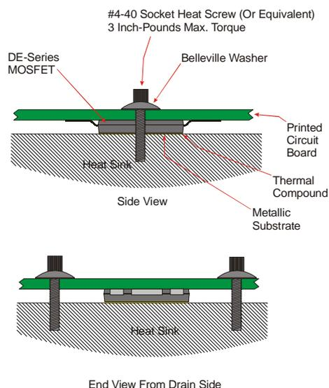
**Figure 2 - EVIC420 Side Views Showing DEIC420 and DE-Series Power Devices Installed In High-Power Configurations<sup>(1)</sup>**
