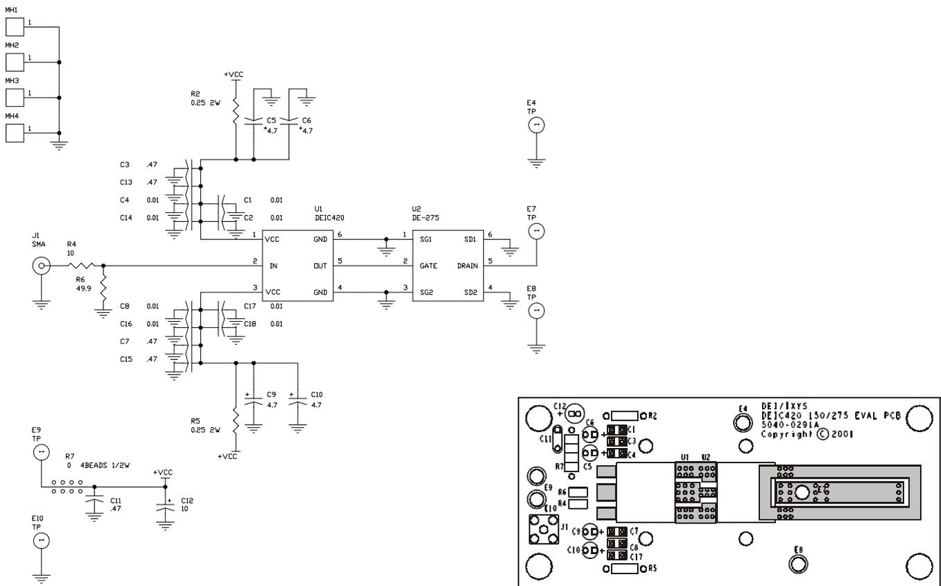
**NOTES:** 1) The schematic shows a DE275 MOSFET, however a DEI DE-150 or DE-275 package type may be installed on the EVIC420-A, and a DE-375 or DE-475 package type may be installed on the EVIC420-B. The EVIC420 is provided without a MOSFET, so that the user can install the appropriate MOSFET for their application. DEI MOSFET data sheets are available on the DEI web site at [www.directedenergy.com/Products/specs/deseries.htm](http://www.directedenergy.com/Products/specs/deseries.htm).
