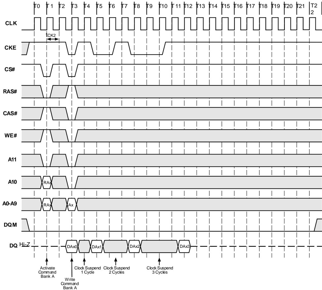
**Figure 7.3. Clock Suspension During Burst Write (Using CKE)**
