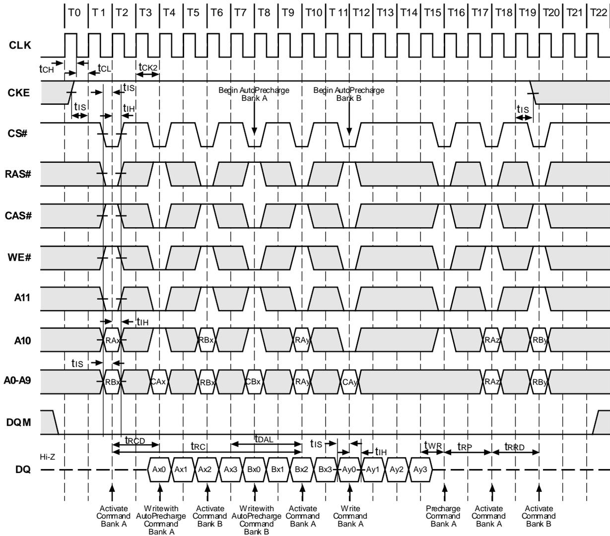
Figure 2. AC Parameters for Read Timing (Burst Length=2, CAS# Latency=2)
