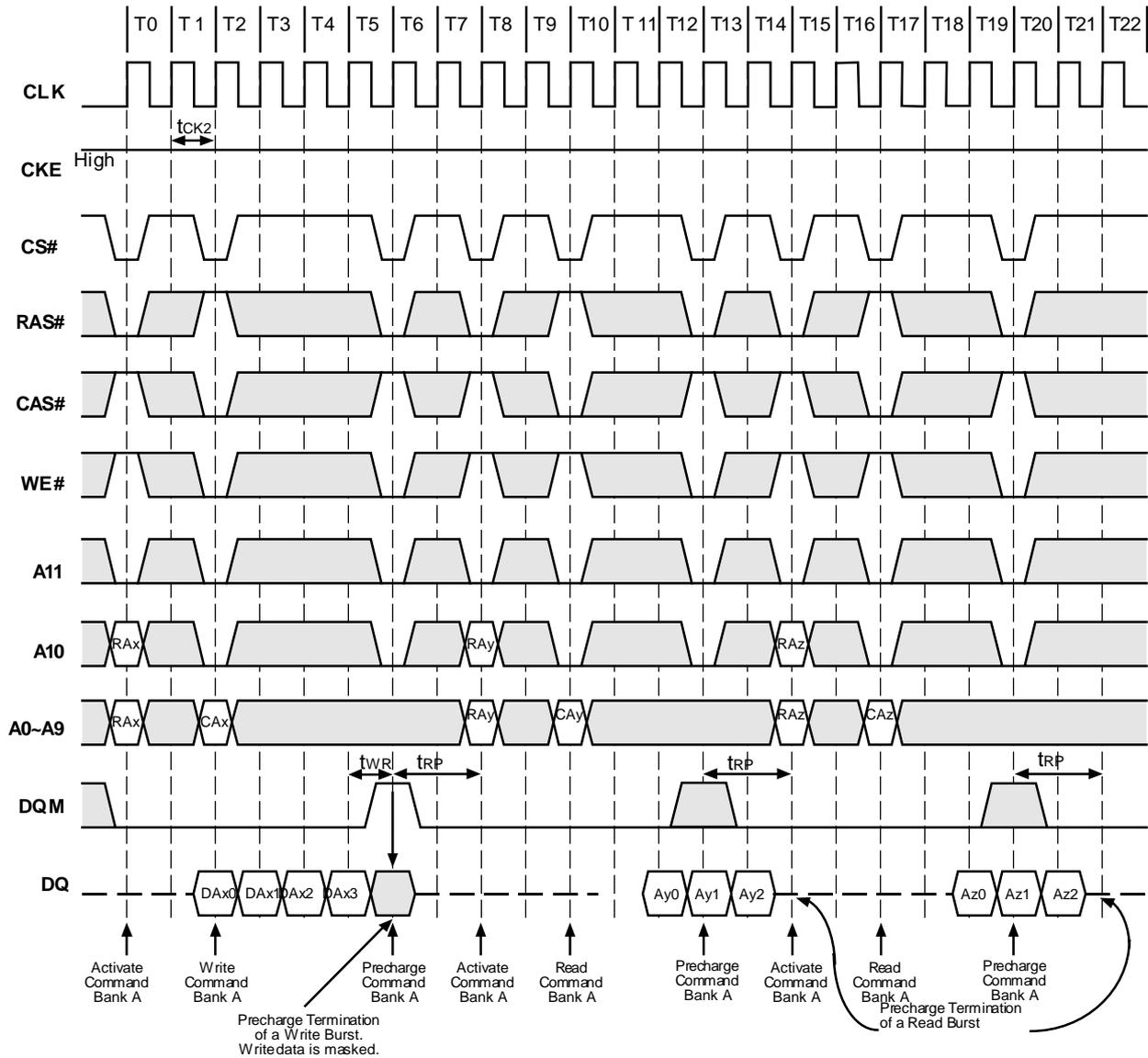
**Figure 24.3. Precharge Termination of a Burst**
