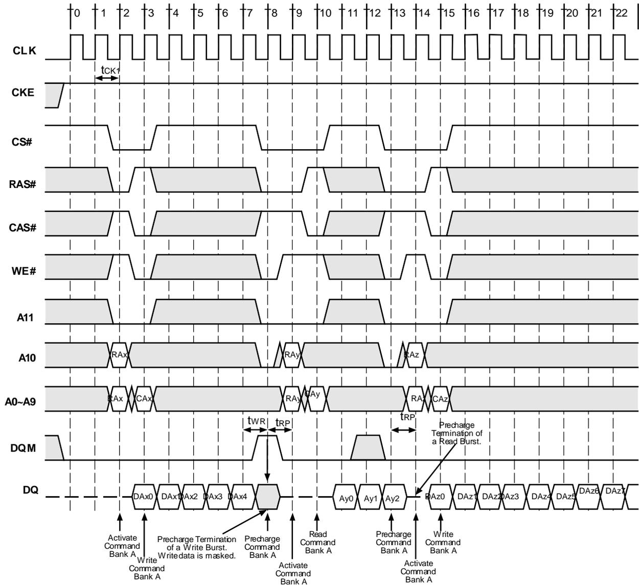
**Figure 24.2. Precharge Termination of a Burst**
