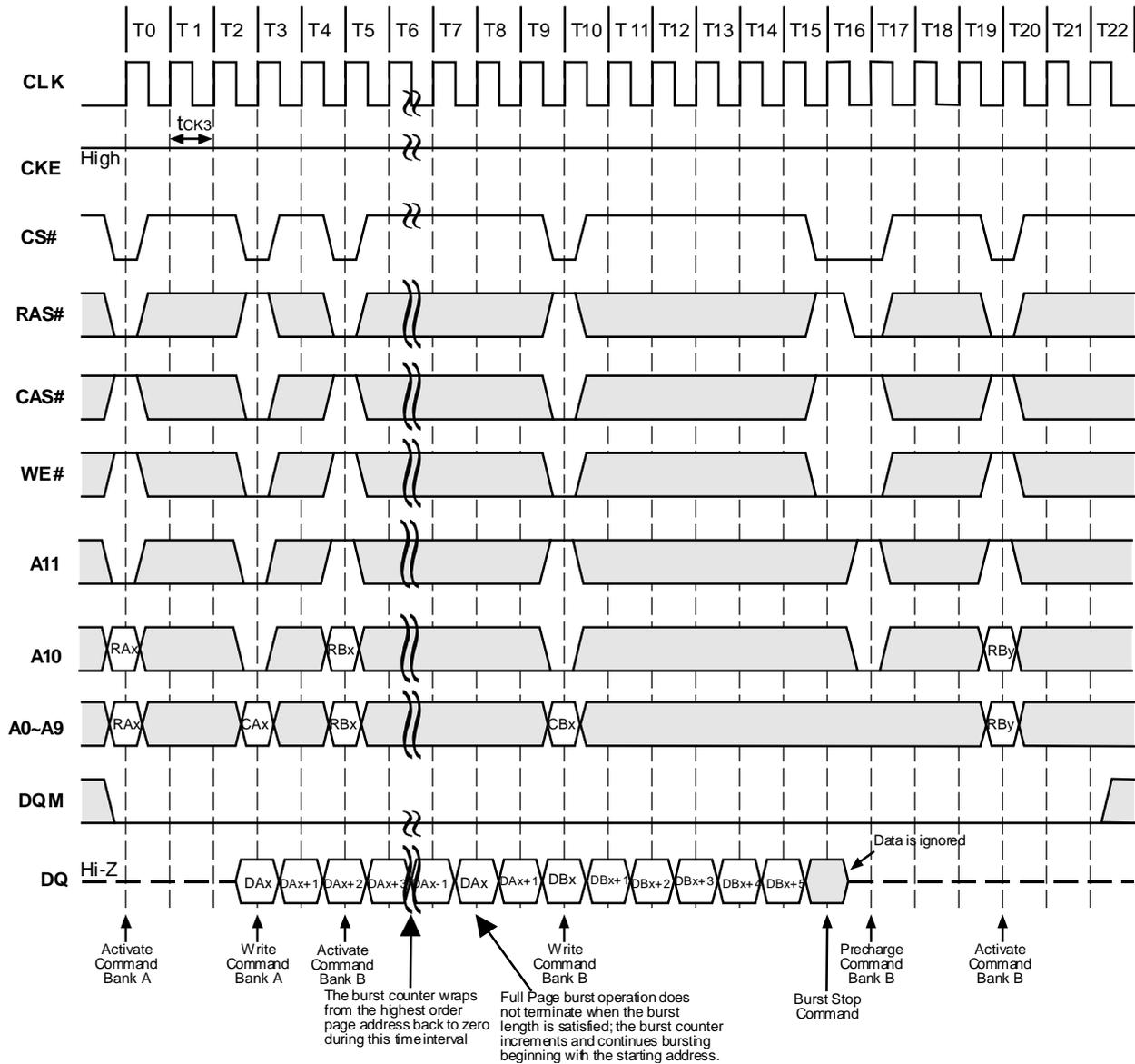
**Figure 20. Byte Write Operation (Burst Length=4, CAS# Latency=2)**
