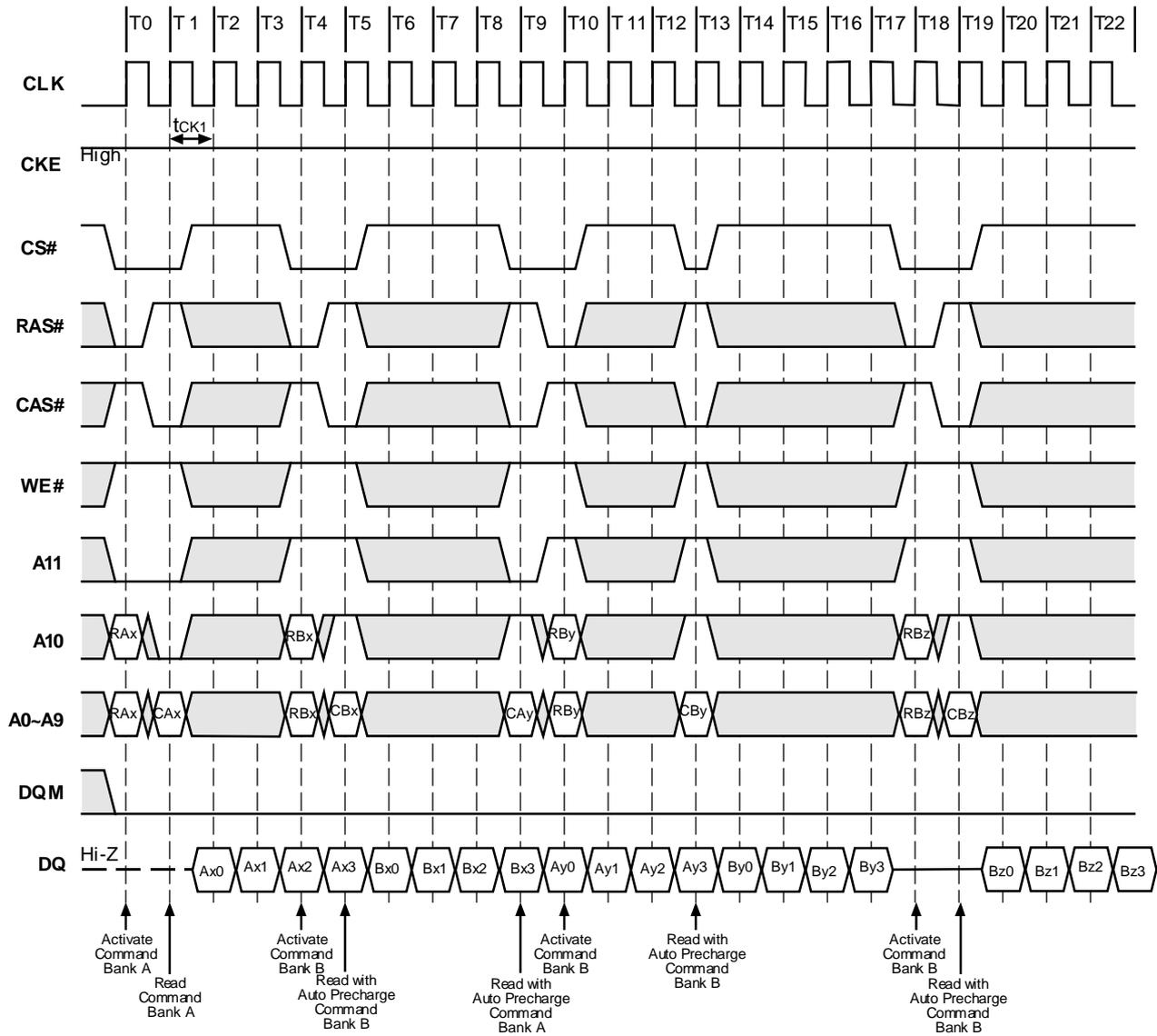
**Figure 16.2. Auto Precharge after Read Burst (Burst Length=4, CAS# Latency=2)**
