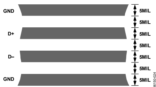
Figure 24. Typical Arrangement of Signal Tracks
