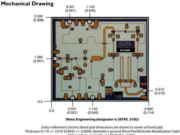
All Bond Pads are 0.100 x 0.100 (0.004 x 0.004). Bond pad centers are approximately 0.109 (0.004) from the edge of the chip. Dicing tolerance: +/- 0.005 (+/- 0.0002). Approximate weight: 4.491 mg.
