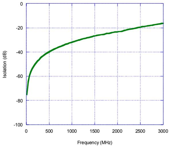
**Figure 11. Isolation – RF1 to RF2, RF2 to RF1**
