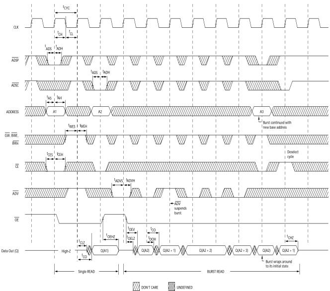
**Note:** 23. On this diagram, when  $\overline{CE}$  is LOW:  $\overline{CE}_1$  is LOW,  $CE_2$  is HIGH and  $\overline{CE}_3$  is LOW. When  $\overline{CE}$  is HIGH:  $\overline{CE}_1$  is HIGH or  $CE_2$  is LOW or  $\overline{CE}_3$  is HIGH.
