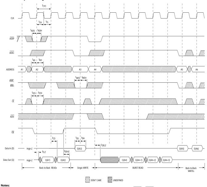
25. The data bus (Q) remains in high-Z following a Write cycle, unless a new Read access is initiated by ADSP or ADSC. 26. GW is HIGH.
