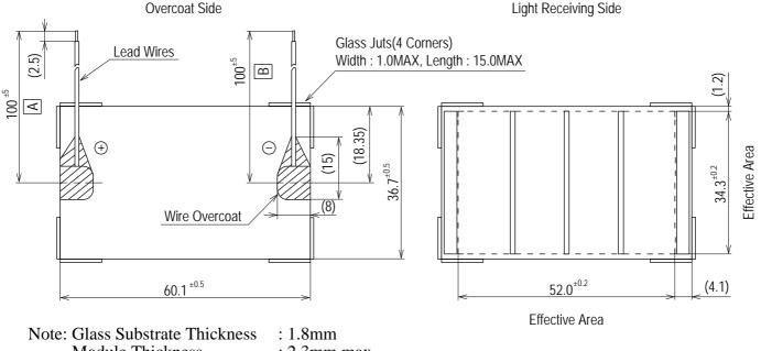
Module Thickness Wire-Overcoat Thickness : 2.3mm max
