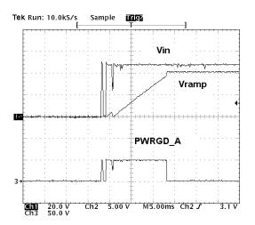
$t_{\text{PWRGD-A}}$  is the time delay from  $V_{\text{EEUV(on)}}$  to PWRGD-A going active. It can be approximated by
