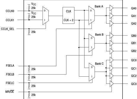
Figure 1. MPC9446 Logic Diagram
