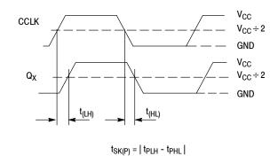
Figure 10. Output Pulse Skew (t<sub>SK(P)</sub>) test reference
