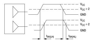
The pin-to-pin skew is defined as the worst case difference in propagation delay between any two similar delay paths within a single device
