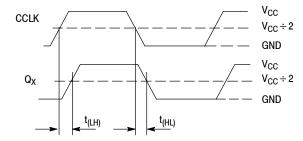
Figure 8. Propagation delay (tpD) test reference
