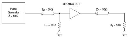
Figure 6. CCLK0,1 MPC9446 AC test reference for  $V_{cc}$  = 3.3V and  $V_{cc}$  = 2.5V
