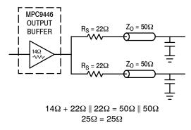
Figure 5. Optimized Dual Line Termination
