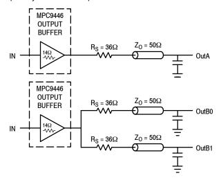
Figure 3. Single versus Dual Transmission Lines
