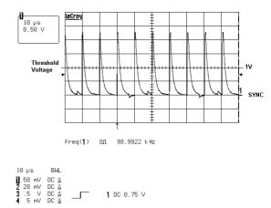
**OUTPUT DRIVES:** The four output drives are designed so that switches A and B, C and D never turn on simultaneously. The OUTA-OUTB pair is intended to drive one half-bridge in the external power stage. The OUTC-OUTD pair will drive the other half-bridge.
