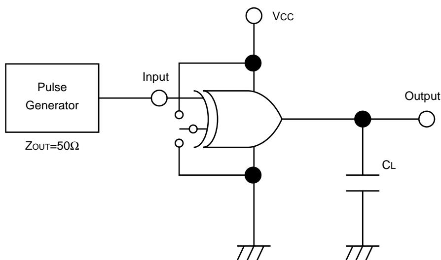
Note: open output when measuring supply current
