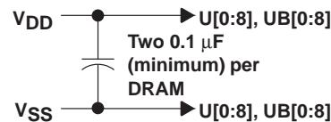
**TM2EP64DPN, TM2EP64DJN, TM4EP64DPN, TM4EP64DJN
