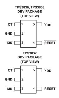
When CT is connected to GND a fixed delay time of typical 10 ms is asserted. When connected to V<sub>DD</sub> the delay time is typically 200 ms.
