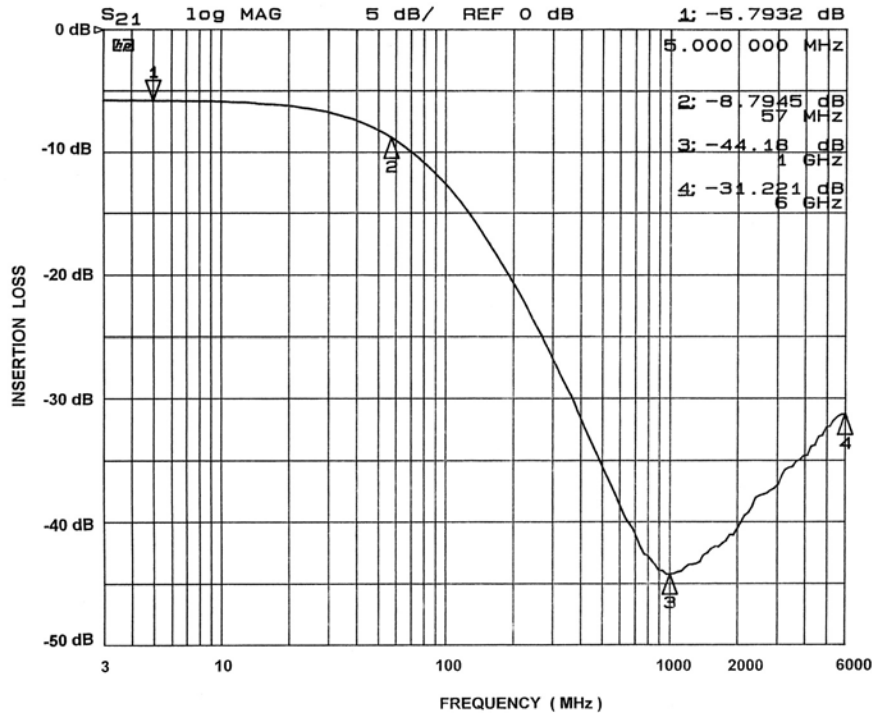
Figure 3. Insertion Loss vs. Frequency (A4-C4 to GND B2)
