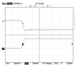
Operating conditions are as follows: Vin=5V, Vo=3.3V, Load change from Io=100% to Io=0%, TA=25°C, Cin=0F, Co=μF.
