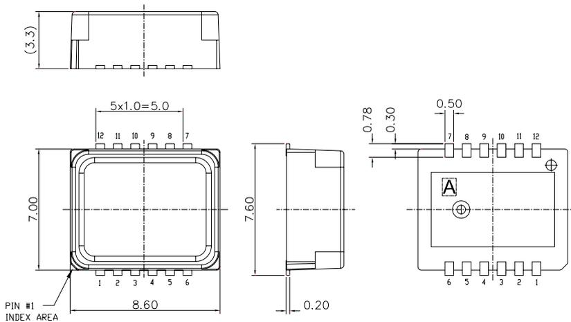
**Figure 3.** Housing dimensions
