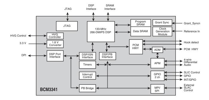
The BCM3341 offers the industry a highly integrated, cost effective approach to developing voice cable modem solutions for the delivery of primary or secondary line telephony. The BCM3341 provides a seamless interface to the BCM3349 single chip DOCSIS/EuroDOCSIS<sup>TM</sup> 2.0 cable modem.
