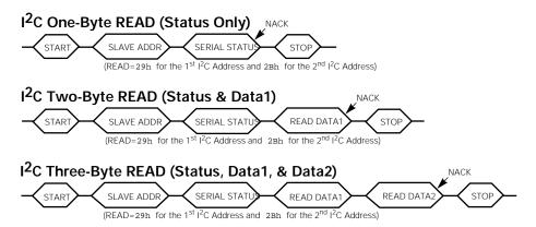
**Note:** In all I<sup>2</sup>C READ operations, the most recent byte read from the Z86230 must be acknowledged by the master with a NACK (Not ACKnowledge).
