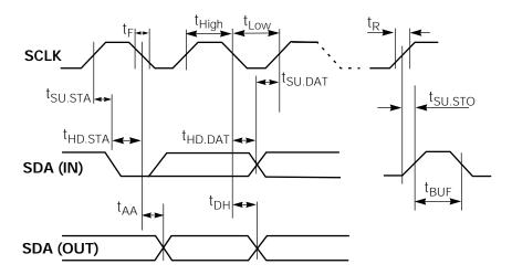
TABLE 6. I<sup>2</sup>C SERIAL TIMING MIN/MAX
