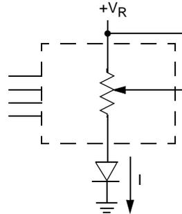
Two terminal Variable Resistor;
