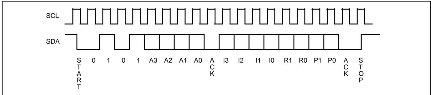
The Increment/Decrement command is different from the other commands. Once the command is issued and the X9258 has responded with an acknowledge, the master can clock the selected wiper up and/or down in one segment steps; thereby, providing a fine tuning capability to the host. For each SCL clock pulse ( $t_{HIGH}$ ) while SDA is HIGH, the selected wiper will move one resistor segment towards the  $V_H$  terminal.
