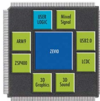
Figure 1. Example of an electronic toy SoC based on the ZEVIO architecture
