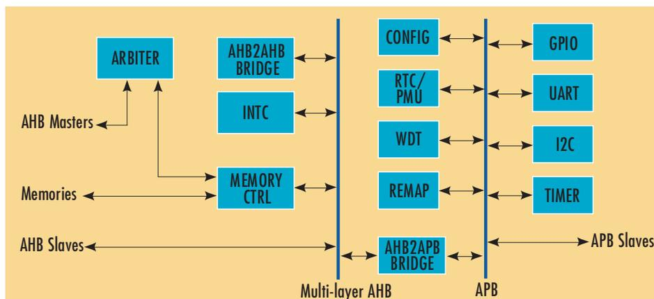
Figure 2. ZEVIO Application Processor Architecture Block Diagram
