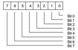
Bit 7 ~ 0: Baud rate divisor latch lower byte values. Default to be 1Fh.
