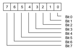
Bit 7 ~ bit 0: Access port for receiver FIFO.
