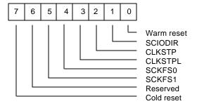
Bit 7: Cold reset. Setting "1" to this bit turns off power to Smart Card interface by pulling up SCPWR#. SCCLK is stopped, SCRST# kept low, SCIO in input mode and SCLED is inactive. ECR's SCIODIR, SCKFS1 and SCKFS0 control bits and control bits in CBR, GTR, BLH and BLL are cleared to default values. User must write a "0" to this bit to recover to normal state.
