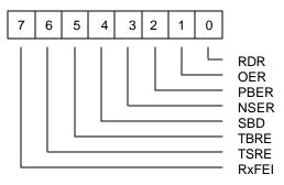
Bit 7: RxFEI means receiver FIFO error indication. This bit is set to "1" when there is at least one parity bit error, no stop bit error or silent byte detected error in receiver FIFO. It is cleared by reading from SCSR if there is no remaining error left in receiver FIFO.
