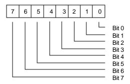
Bit 7 ~ 0: Baud rate divisor latch higher byte values. Default to be 00h.
