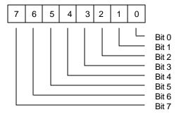
Bit 7 ~ 0: Clock base value. It specifies number of internal sampling clock pulses for a data bit. Default to be 0Ch.
