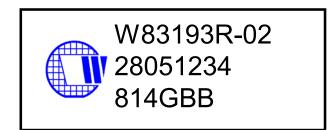
1st line: Winbond logo and the type number: W83193R-02/-04 2nd line: Tracking code <u>2</u> 8051234 <u>2</u>: wafers manufactured in Winbond FAB 2 <u>8051234</u>: wafer production series lot number 3rd line: Tracking code <u>814 G B B</u> <u>814</u>: packages made in '<u>98</u>, week <u>14</u> <u>G</u>: assembly house ID; A means ASE, S means SPIL, G means GR <u>BB</u>: IC revision
