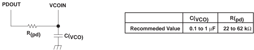
Figure 8. Resistor and Capacitor Connection
