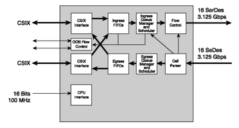
The BCM83XX switch fabric chipset is a highly integrated scalable switch fabric, consisting of the BCM8320 Fabric Interface chip and the BCM8332 Switch chip. The BCM83XX switch fabric is ideal for these applications:
